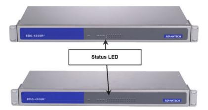
Figure 2.3: EDG-4508R+/4516R+ Front Panel
